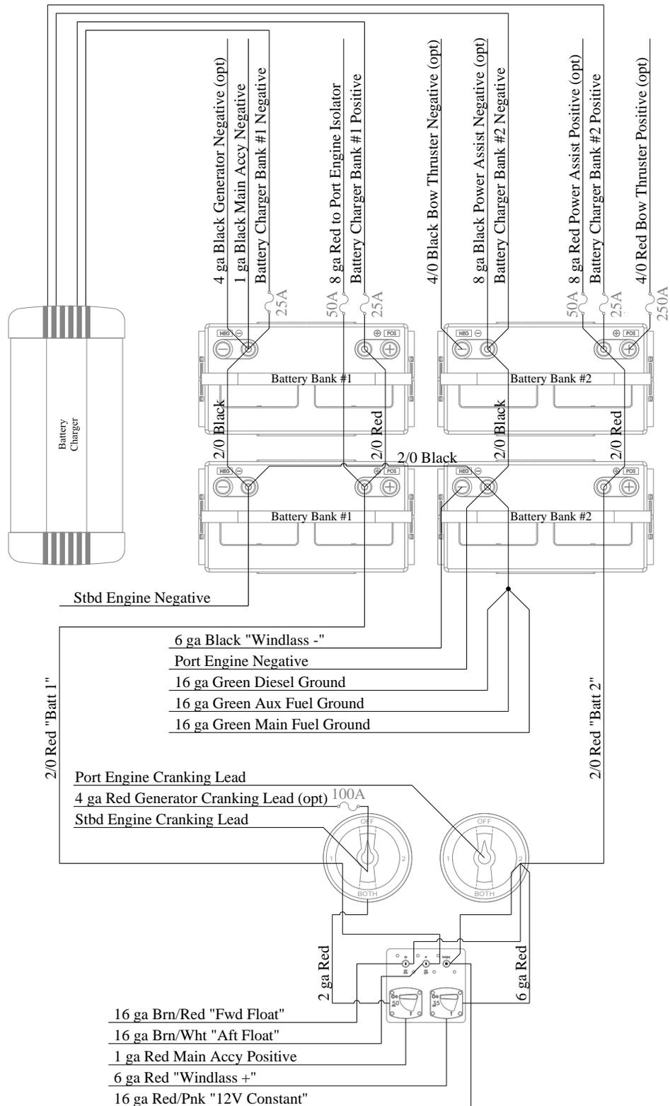
NOTE: 50A engine isolator fuse changes to 100A MRCB if the boat is equipped with V6 engines.
